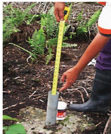
How to measure the difference of peat water level on peat land (Suryadiputra et al., 2005)
