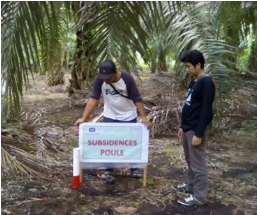
Simple instrument to measure peat subsidence
