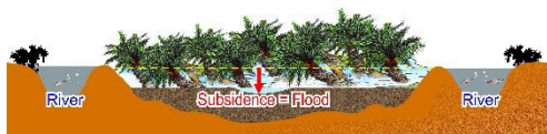
Subsidence in oil palm plantation (top, Winrock Int.); subsidence illustration of oil palm plantation on peat (bottom: WII)
