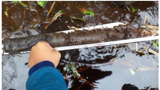
Peat depth measuring tool / drill (Winrock Int.)
