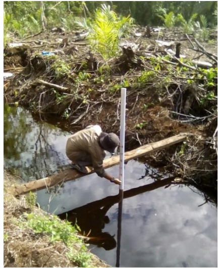
The ruler of water level in the drainage/weir (left); and the daily measurement activity (right)
