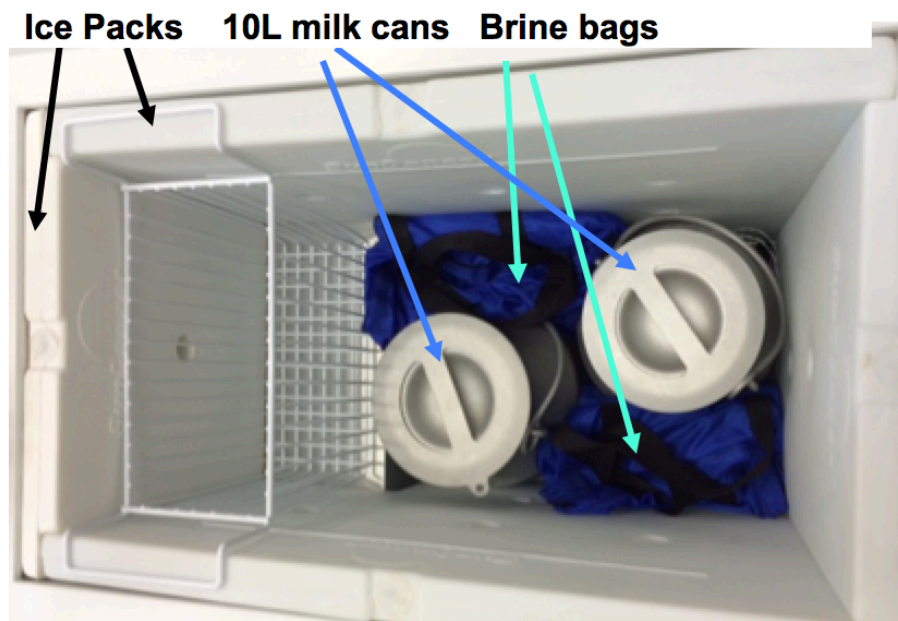
Fig. 3: PV using thermal ice storage and brine bags to chill evening milk.
