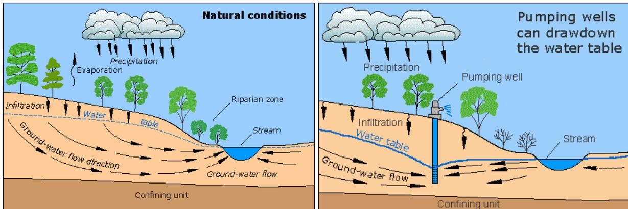
Figure 5. Interaction between surface and groundwater. Source: <https://water.usgs.gov/edu>
